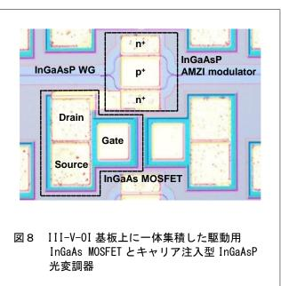
Electronic-photonic integrated circuits based on III-V photonic-wire waveguides
